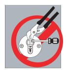
**NEVER** use additional tools or objects to create extra torque to rotate the key
