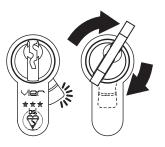
Rotate key to align cam with cylinder body to allow installation
